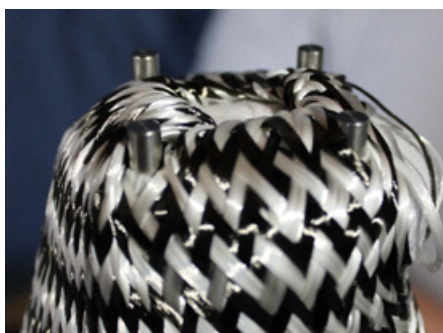
Example of loose tie off of braid to Perl or flexastretch (sew end) (Can put Dacron Felt first layer if needed)
